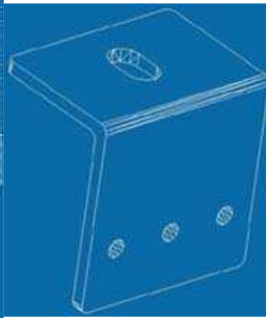
Connecting Fitting of Column
